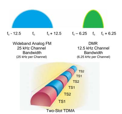
For the amateur, this means one repeater allows two separate channels at the same time. Currently most amateur DMR repeater system implementations utilize both channels for voice and some limited text messaging. Typically one channel (time slot) is used for wide-area and the second is local and regional Talk Groups.
